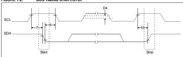
FIGURE 1-2: BUS TIMING START/STOP
